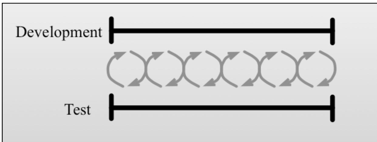
When test and code writing are integrated, we prevent defects. Not all defects, but many of them. This process is designed to prevent defects, and it has a profound effect on design and how we spend our time.
