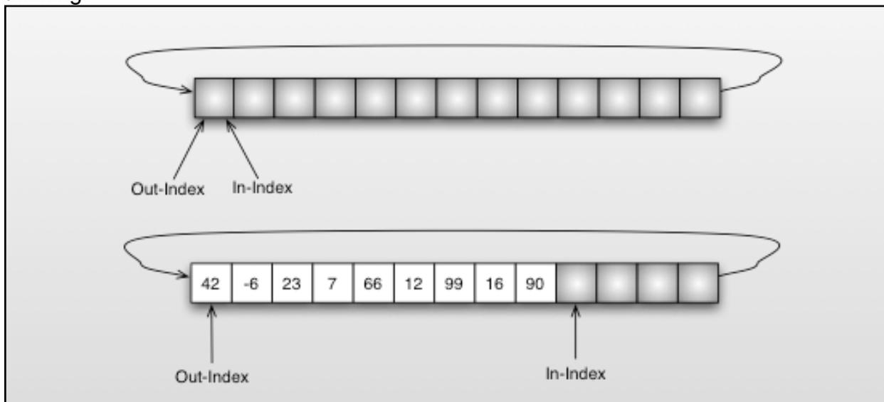
We can anticipate that we will need two indexes. For the current tests a single index will do. If the index is zero, the buffer is empty (at least for our current test scenarios). Following the state machine, we'd add the interface and see the link error, then add an empty implementation for `CircularBuffer_Put` and watch the test fail. I'll leave that to your imagination this time. Here is the minimal implementation that makes both the tests pass:
