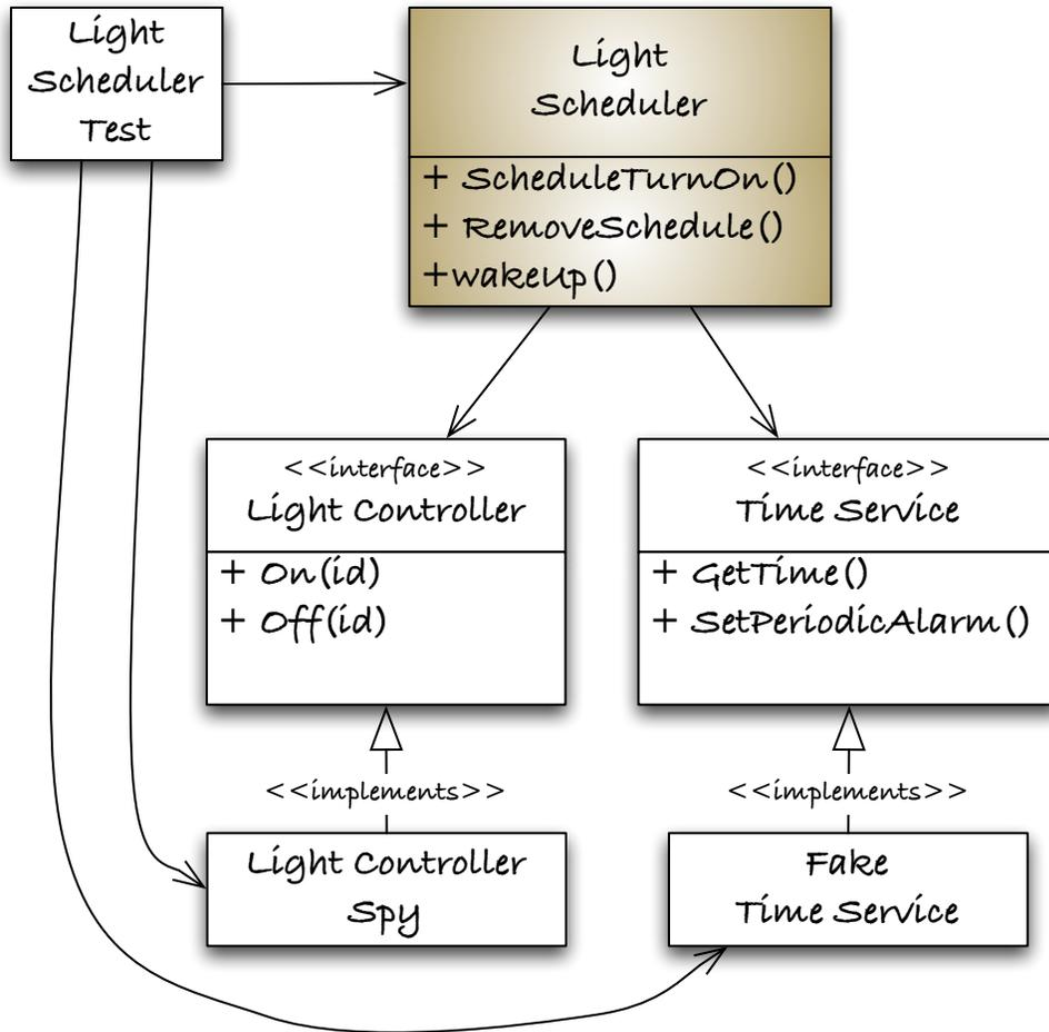
The test case takes the place of the client of the LightScheduler. The FakeTimeService replaces the TimeService during test as the LightControllerSpy does for the LightController. The LightScheduler has no idea that it is not working with test versions of its collaborators.
