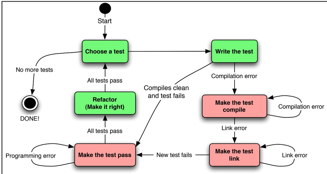
After writing the test and compiling, we are at the “Make the test compile” state. That makes us add the `CircularBuffer_IsEmpty` function prototype to the header file, like this:
